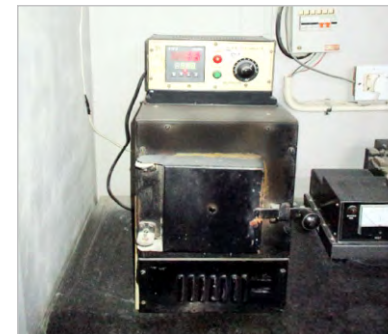
Muffle Furnace MSFRT-3 Range: 0°C to 1000°C
